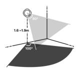
2.2.5 Notice The height of SiMP Motion Sensor must be higher than 1.6 meters from the ground. If
